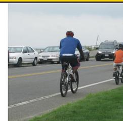
A paved extension of the road's shoulder outside of the motorized vehicle travel lanes.
